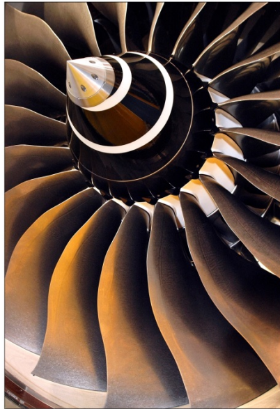
The swept fan of the Trent 1000 contains only 20 blades
