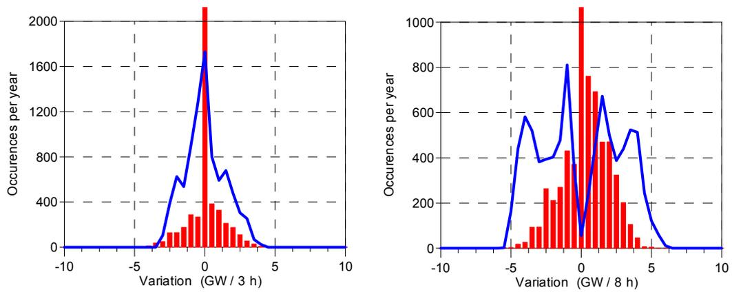
Figure 3.20. Total load variation (cont. lines) and residual load after full exploitation of the PHESS system (bars), for 80% scenario – case A.
