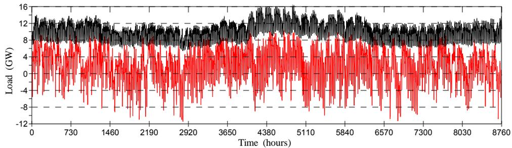
Figure 1. Load (black) and Residual Load (red) for the 80% RES scenario - case A.
