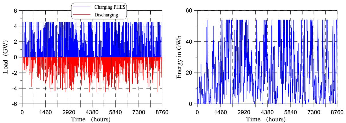
Figure 3.16. Power and charging level of PHEs system only for RES storage – case A.
