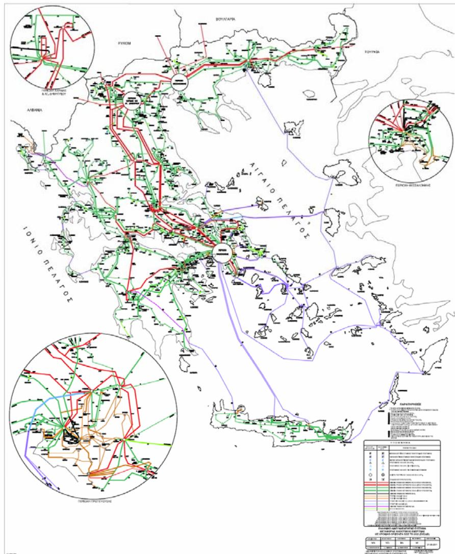
Figure 1.5. Transmission lines after interconnection of the Aegean Island ([www.admie.gr](http://www.admie.gr))
